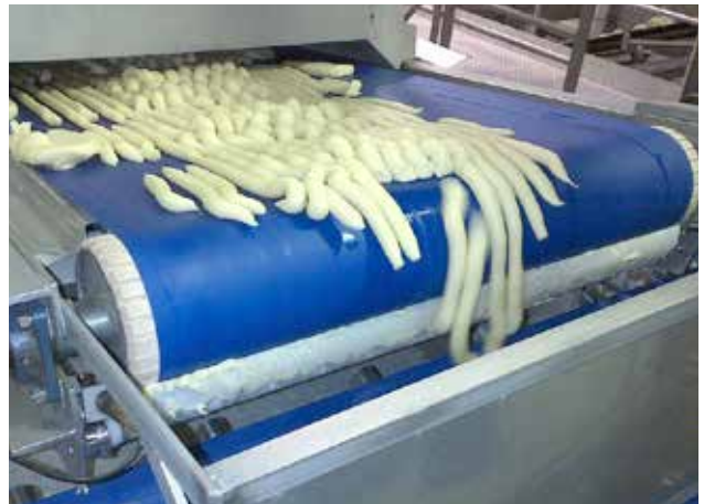
Fries conveying after frying
