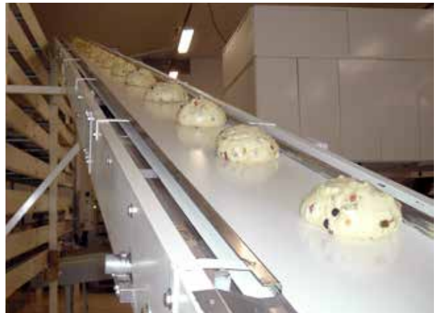
Inclined conveying towards multistory open air proofer
